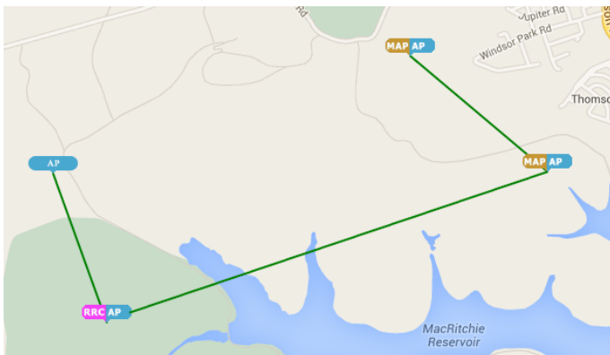
Figure 61: An existing AP is connected to an RRC which is in turn connected to 2 MAPs.
