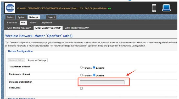
INPUT 250 IN ABOVE POSITION, THEN SAVE AND APPLY. Both AP(WDS) mode and Client(WDS) mode support.
